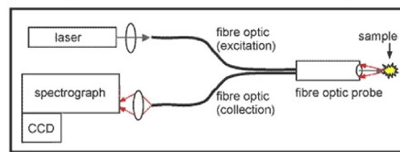
The basic components for Raman spectroscopy include a light source (normally a laser), collection optics to gather the Raman-scattered light, and a detection system. The detector is the heart of the system. It must be able to filter out stray light signals that may prevent the Raman peaks to be seen. Multiple dispersion stages are employed to reduce the amount of this stray radiation. A CCD camera is used to detect the Raman shifted light.
