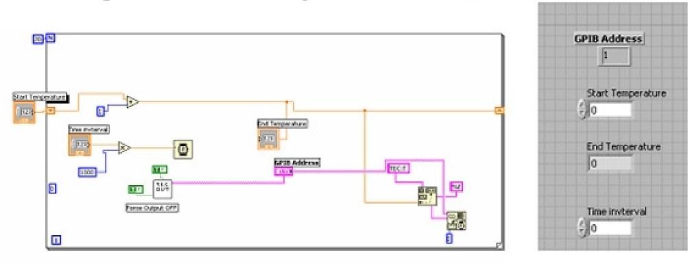
A program that invovles taking the data from the Keithley 2000 Multimeter and writing it into a file.
