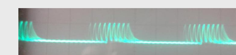
Figure 6 Output of the ADG1236 [6]
