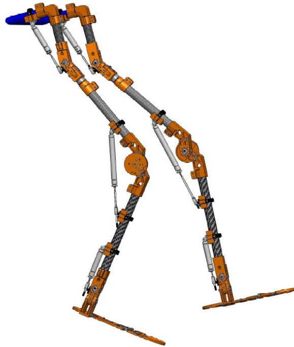
Figure 1. Solidworks of the lower limb exoskeleton prototype.
