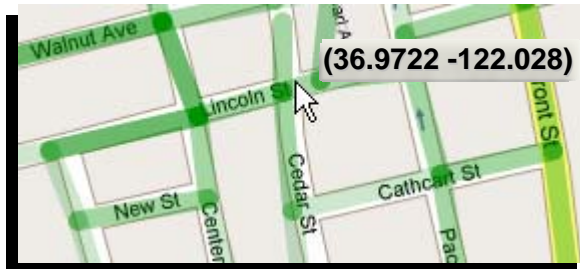
Figure 3: The cursor is at the latitude-longitude coordinate (36.9733, -122.028), which is sent to the Geonames database to get more street information. This process of gathering data from a coordinate is called reverse-geocoding.
