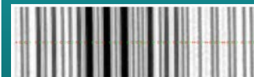
Fig 5. Final Result. The left side of each bar is marked with a red circle, the right side with a red circle, and noise is marked with red crosses
