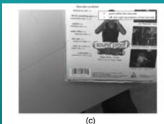
Fig 3. (a) The original image (b) Equation 1 is applied to the image, and the result is low-pass filtered. The red region, which is of the highest intensity, corresponds to the barcode. (c) The barcode is localized using image b). Left and right barcode boundaries are determined.
