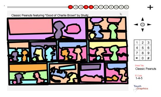
The TTT authoring tool allows the user to add audio to different regions. To do so, the author must mark the vertices of each region manually and either type for text-to-speech or include an audio file. There is an option to record audio in the TTT, but the volume remains very quiet using this.
