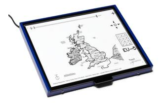
The Touch Tactile Tablet (TTT) is a large, touch screen input created by Touch Graphics<sup>2</sup>. Designed for visually impaired users, TTT links audio data to areas of the touch screen's surface.
