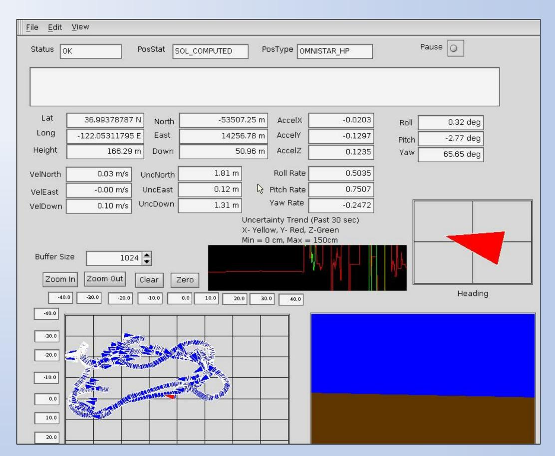
The NAV VIEWER maps position, pitch, roll and yaw data. The recorded data can then be analyzed back in the lab, to asses how well the vehicle navigated the course.
