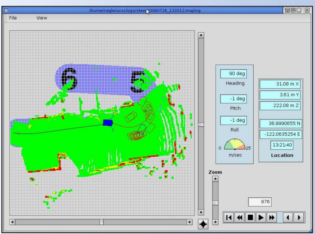
The SiCK LiDAR is used to generate a map of the surrounding area, color coded to indicate the traversability of the terrain.
