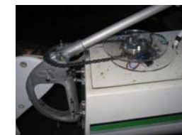
Completed Motor Control Subsystem Mounted in Boat Hulls
